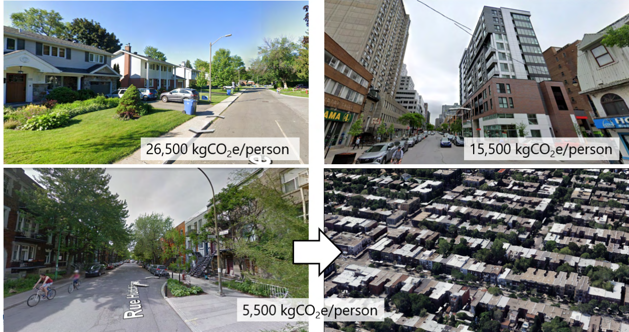
Figure 1 – Example of embodied GHG emissions in neighbourhoods per capita (if they were built today).
