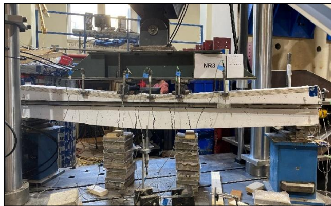
Fig. 1—Short-term flexural test - NR3 [ h = 300 mm].
